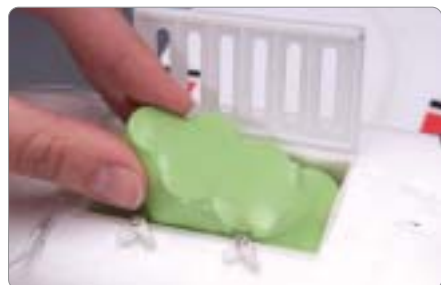
When installing the battery pack, be sure to stick the connector all the way into the small opening in the compartment. This ensures that there's room for the battery pack to fit properly, and you'll be able to close the hatch and secure the thumb tabs that hold the hatch shut.
