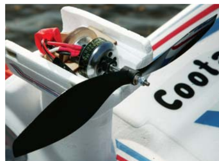
The brushless motor and ESC are both mounted in the pylon. The cowl is also retained with magnets.
