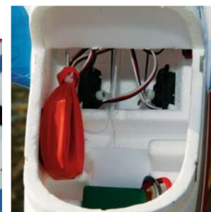
The servos and receiver, sealed in a balloon, are easily accessible through the main cockpit. The cover is retained with rare earth magnets.
